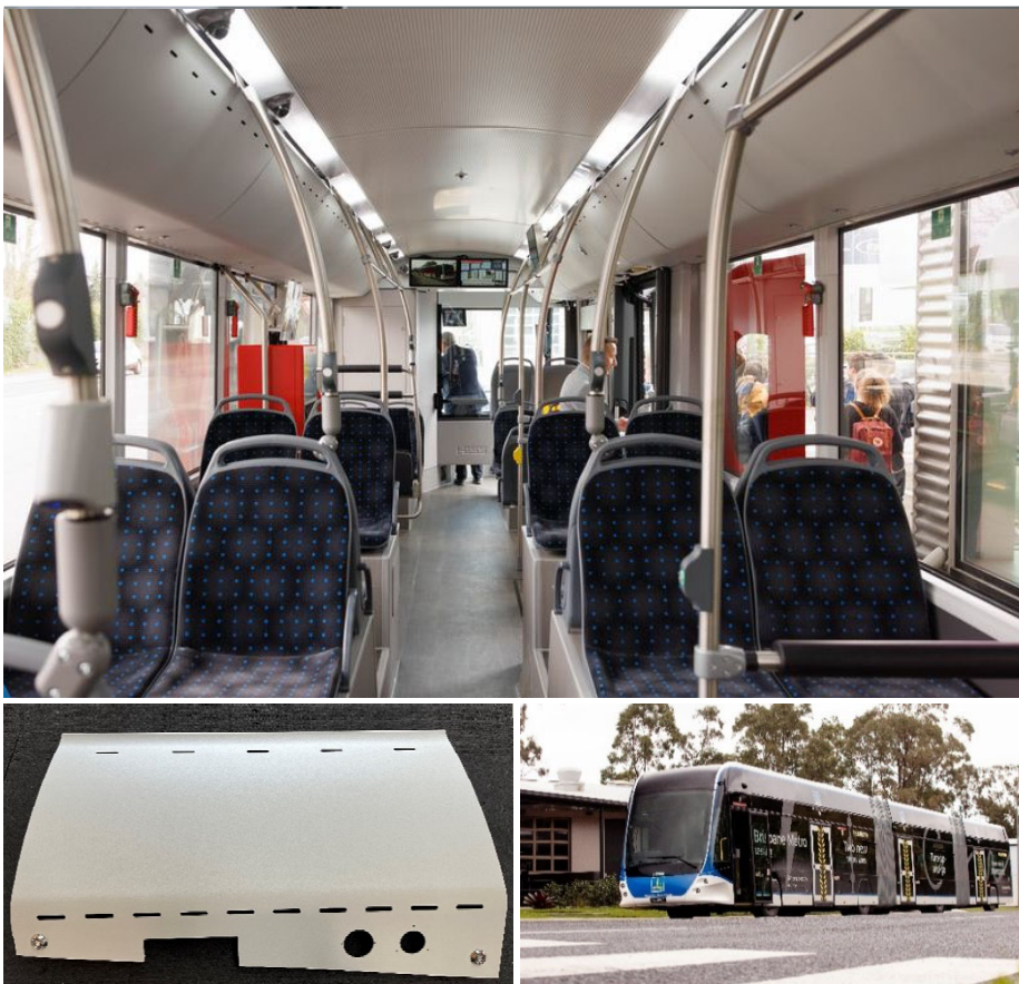
Top: interior view of the electric bus; bottom left: thermoformed roof frame cover made of SIMORAIL HL3; bottom right: exterior view of the electric bus
